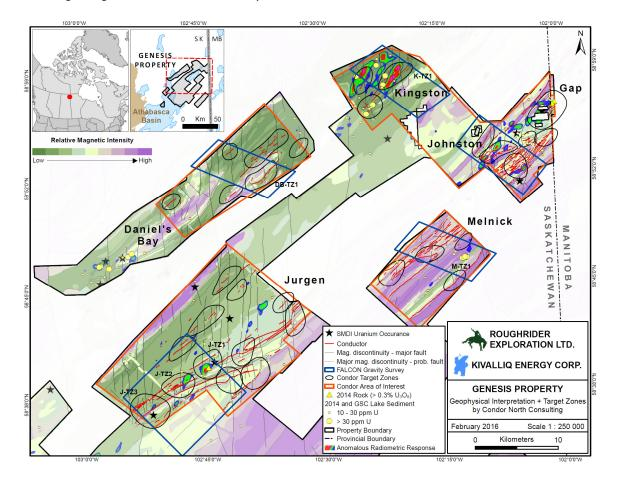
In February and March of 2016 a 1,677 line-kilometre fixed-wing FALCON airborne gravity gradiometer (AGG) survey was completed on the Genesis property by CGG Canada Services Ltd. Independent review of the data was provided by in3D Geoscience Inc. The AGG survey was divided into five survey grids to cover previously highlighted priority areas: Jurgen, Daniel's Bay, Melnick, Kingston and Johnston. Final deliverables were received on April, 8 2016.
