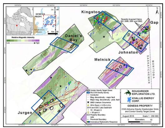
Interpreted FALCON gravity gradiometric low response anomalies.
