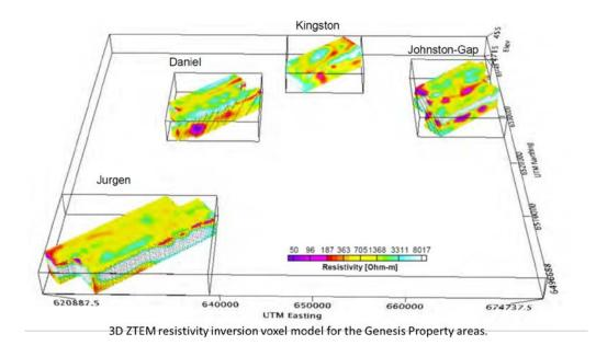
Well defined, generally northeast trending conductors are evident in the survey areas. Resistivity zones are very sharp, especially in the Johnston/GAP area. Significant disruptions are also noted along the trace of some of the conductors, most notably at Jurgen. North trending cross structures are also suggested at Jurgen, Daniel's Bay and Johnston/GAP.
